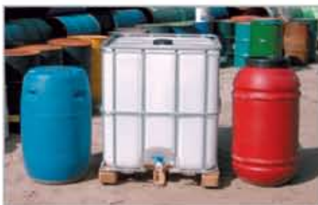
Some common containers used for rain barrels are (left to right): 50-gallon sealed barrel, 275-gallon juice container, 50-gallon open-top barrel.
